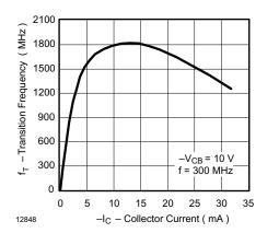
Figure 2. Transition Frequency vs. Collector Current
